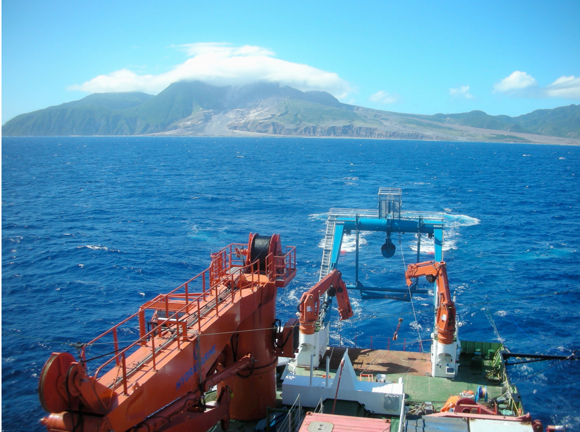
2394 Fig. 24. Shooting on a radial track offshore eastern Montserrat. Airgun 2395 explosion bubbles may be seen behind the hoist. The Tar River valley 2396 leading up to the Soufriere Hills Volcano is in the distance with the volcano 2397 summit covered by cloud cap. Sparks photo. 2398
