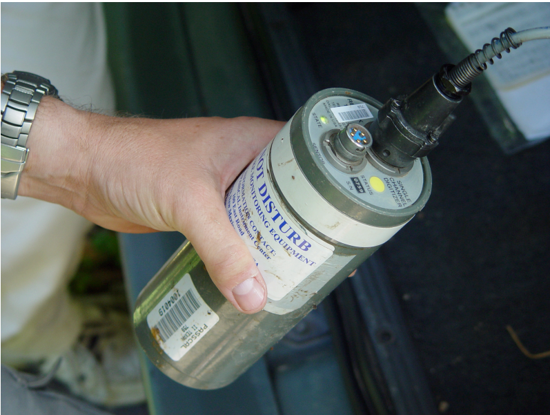
Fig. 8. The RefTek RT125A seismometer, with cable to a single vertical component Mark Products L40 (or L28) 4.5 Hz sensor. B. Voight photo.
