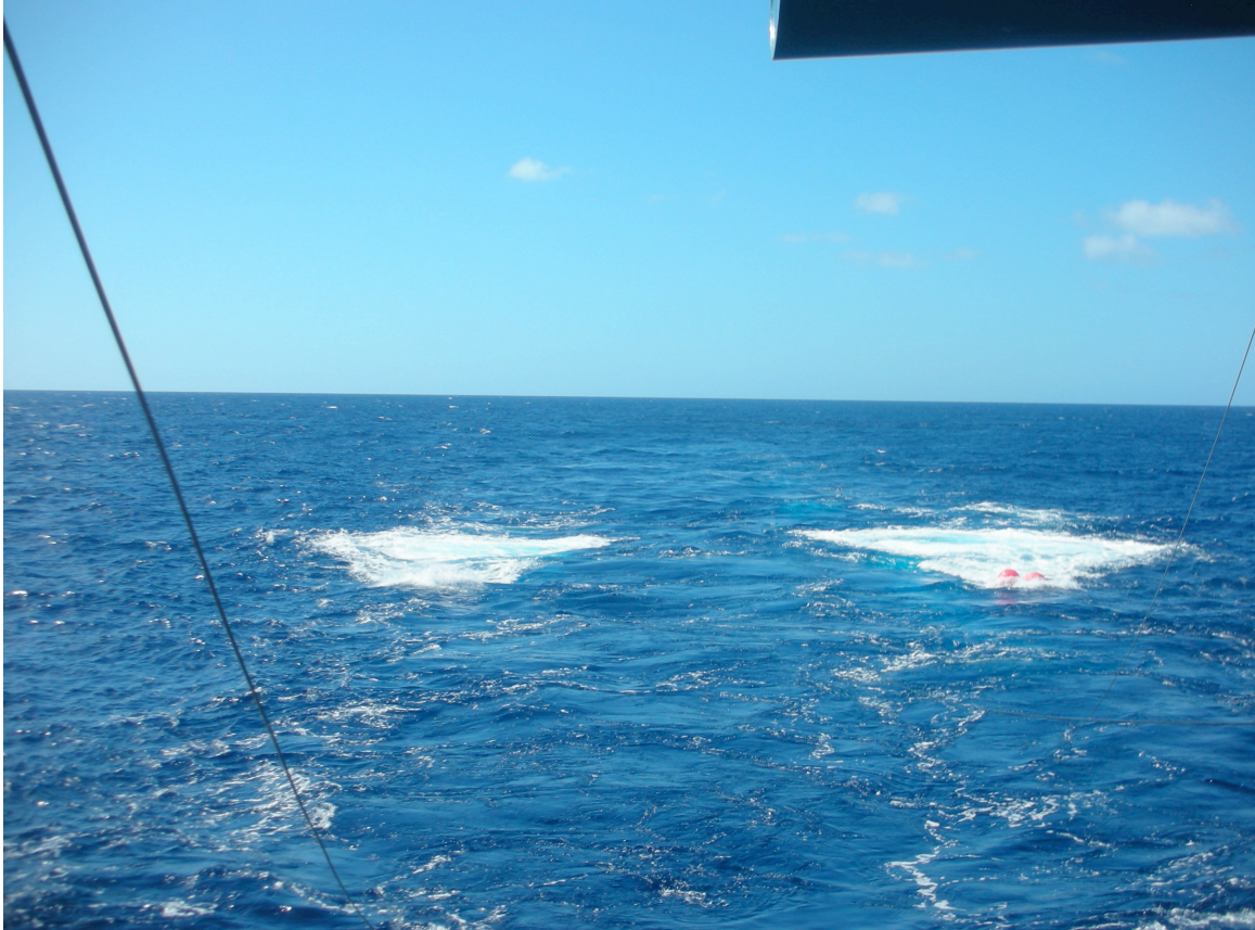
Fig 25. Synchronized explosions from the dual airgun clusters, offshore Montserrat.
