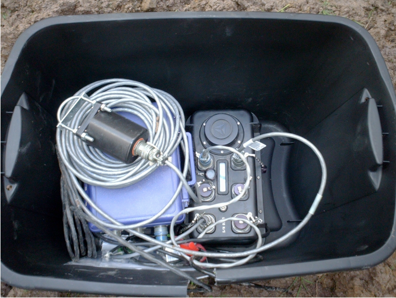
Fig. 7. The RefTek RT130 seismometer recorder, with 3-component Mark Products model L22, 2.0 Hz geophone. B. Voight photo.
