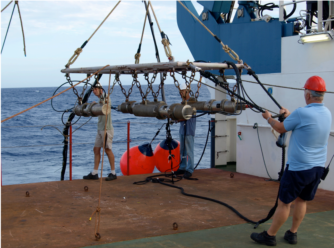
Fig. 23. Airgun array being prepared for deployment off the stern of the RRS James Cook. J. Hammond photo.
