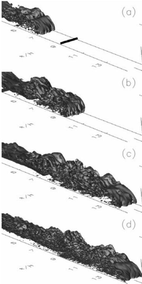
Figure 10. Temporal evolution of a gravity current flow over a cylindrical obstacle such as a submarine pipeline (from Gonzalez-Juez et al. 2009).
