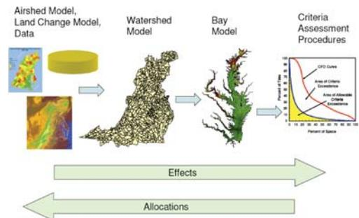
Figure 3. The CBP suite of models. The Airshed model generates nutrient deposition for the watershed model that then calculates the loads that go into the Estuary model.
