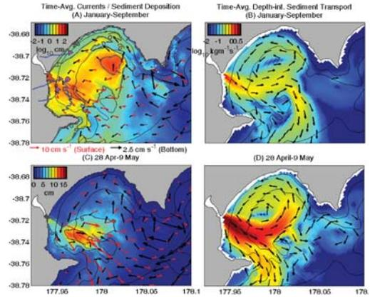
Figure 7. (A, C) Time-averaged currents (arrows) and sediment deposition (colors) over the time frame in the titles. (C, D) Depth-integrated and time-averaged sediment transport direction (arrows) and magnitude (colors), showing the estimated direction and magnitude of sediment transport from the Waipaoa River mouth during 2006. April–9 May encompasses a moderate storm (from Bever et al., 2009).
