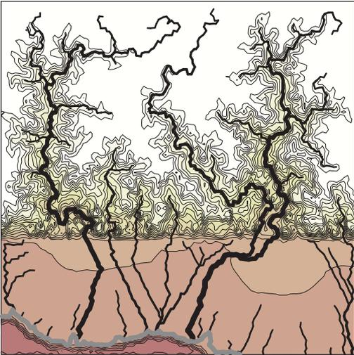
Figure 1. Example simulation using the CHILD landscape evolution model (Tucker et al. 2001), showing erosion of a rising source terrain and growth of fan delta complexes on a subsiding fault block. Domain size is  $10 \times 10$  km.
