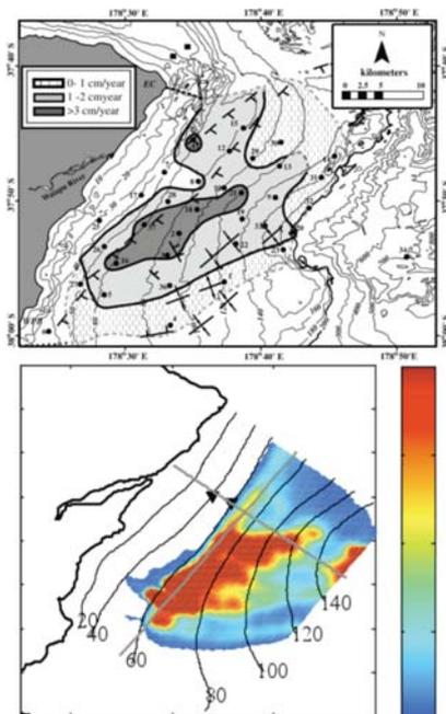
Figure 8. Comparison of observed shelf mud deposits with those predicted by the WSGFAM model for the Waiapu shelf, northeastern New Zealand, for (a) observed  $^{210}\text{Pb}$  sediment accumulation rate (Kniskern et al., in press) and (b) modeled deposit thickness from winter 2004 floods (Courtesy of C.T. Friedrichs).
