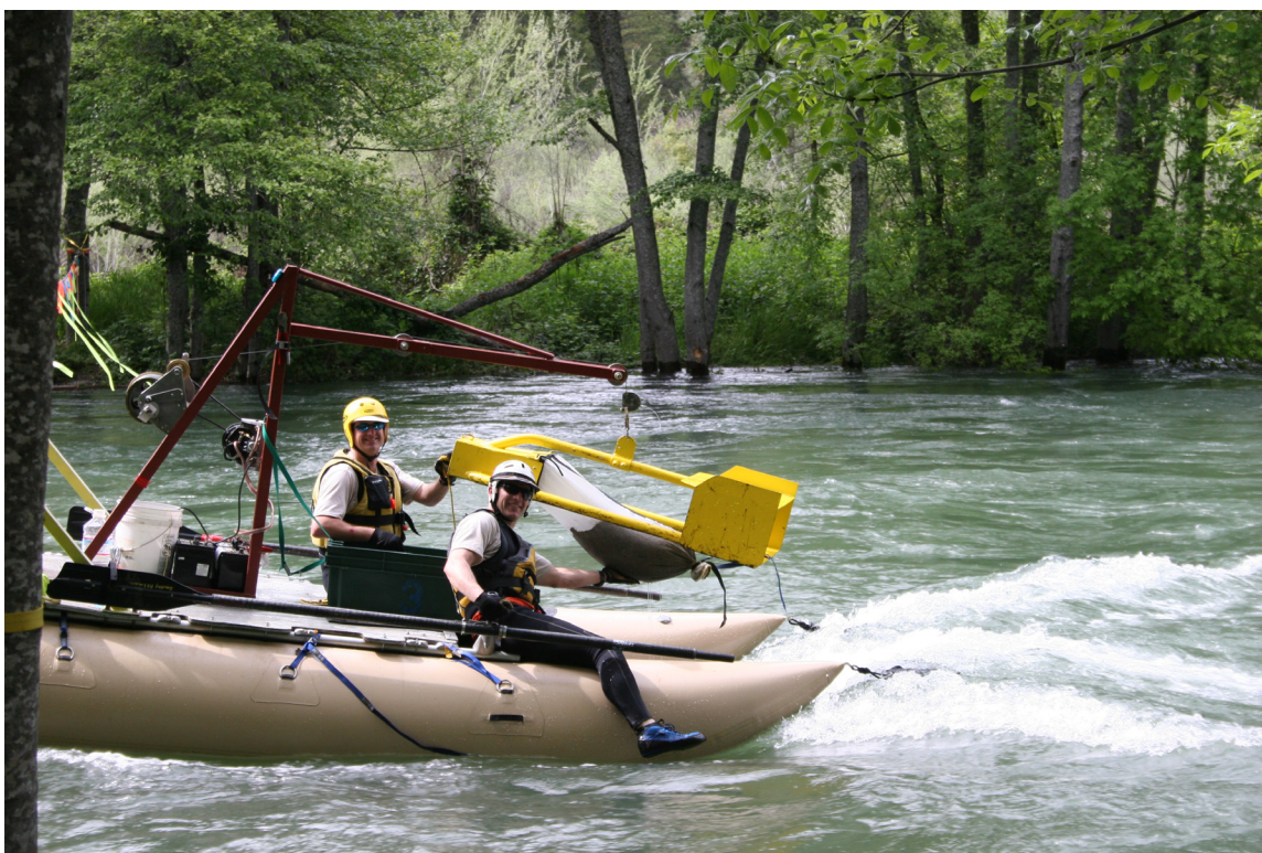
Figure 7-4: Cataraft-based bedload sampling with the TR-2 sampler. Streamers show the location of the cable to which the cataraft is tethered. Photo by the author.
