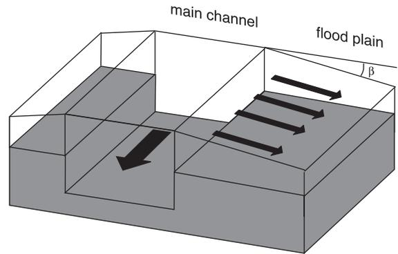
Fig. 10. Schematic diagram of conceptual model of levee formation by advection of suspended sediment. Figure shows the angle of water surface slope ( $\beta$ ) that drives water and sediment away from the main channel. The slope arises from the difference in elevation between the main channel water surface and that of the flood plain.
