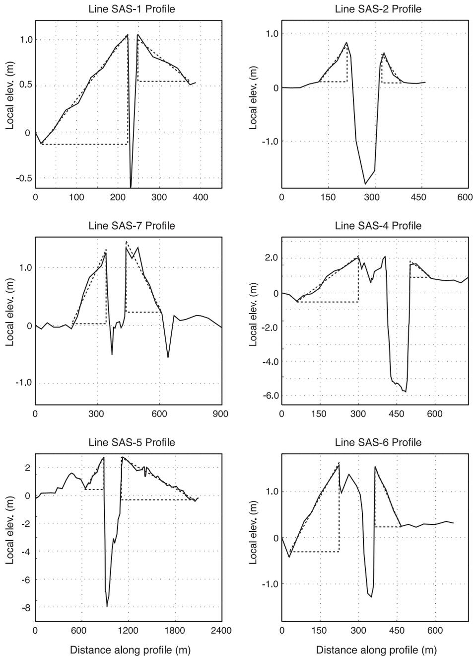
Fig. 4. Cumberland Marshes channel and levee profiles taken from PFRA (1954) surveys. Elevations are reported as meters above mean sea level. Levees have relatively gentle slopes and broad widths typically several times channel width.
