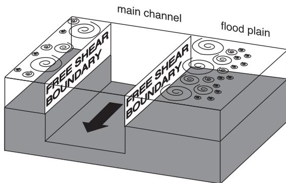
Fig. 9. Schematic diagram of conceptual model of levee formation by turbulent diffusion of suspended sediment. Turbulent eddies form by the interaction of the swiftly moving water of the main channel with the relatively stagnant water of the flood plain. Eddies carry sediment away from the main channel and deposit successively finer sediment with distance into the flood plain.
