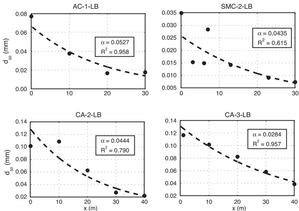
Fig. 7. Surface grain size ( $d_{50}$ ) fining curves for two natural levees of the Columbia River (top) and two natural levees of the lower Saskatchewan River (bottom). The left edge of the plot is the channel margin and the dashed lines are exponential fits to the data of the form of Eq. (1). R-squared values ( $R^2$ ) and fining exponents ( $\alpha$ ) are shown in the text block of each plot. Saskatchewan River data are from Cazanacli (1997).
