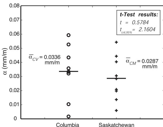
Fig. 8. Comparison of spatial fining rates of levees of the Columbia and Saskatchewan Rivers. Each data point represents the fining exponent of a single levee and solid lines indicate value of mean fining exponent for levees of each site. Results of the  $t$ -test, given in the text block, show that the mean fining rates of the two sites ( $\alpha_{CV}$  and  $\alpha_{CM}$ ) are statistically insignificant at the 95% confidence level.
