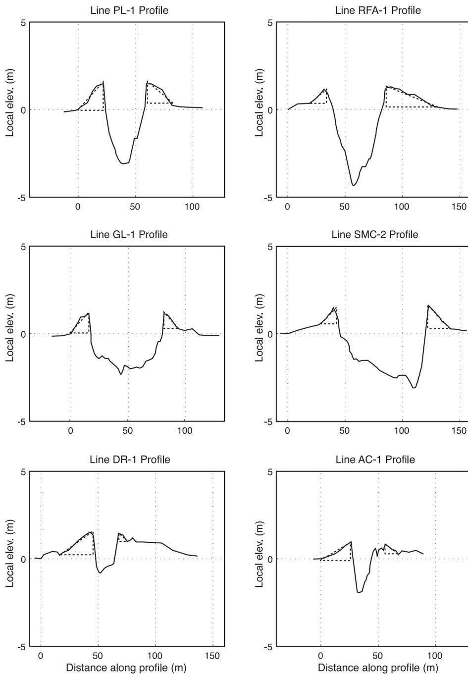
Fig. 3. Columbia River channel and levee profiles. Zero elevation datum is established as the left bank floodbasin elevation, and zero horizontal distance is set at the end of the left bank levee. Levees are relatively steep and narrow, with levee width typically less than channel width. All views are looking downstream.
