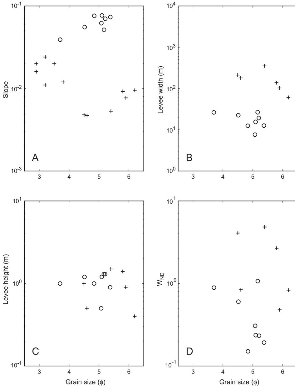
Fig. 6. Morphometric comparison plots for natural levees of the Columbia River (shown in circles) and the Saskatchewan River (shown in crosses) using levee crest mean grain size ( $d_{50}$ ) as the independent variable. Note lack of grain size control on levee morphology at both sites. Data are given in Table 1.
