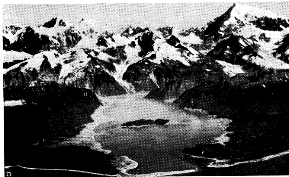
Fig. 33. (a) Lituya Bay, 1954. Trimlines of 1936 giant waves of unknown origin ( g ) and 1853–1854 ( k ). Lateral moraines ( m ) and end moraine in foreground record recent advance of ice to bay mouth. (b) Lituya Bay, August 1958 (after Miller, 1960). Wave generated on July 9 by rockslide ( r ) destroyed forest to maximum elevation 524 m at d and to a maximum distance of 1100 m in from high-tide shoreline at Fish Lake ( F ). Fishing boat anchored at b was carried over spit; boat at entrance was sunk, and boat at e rode out the wave.
