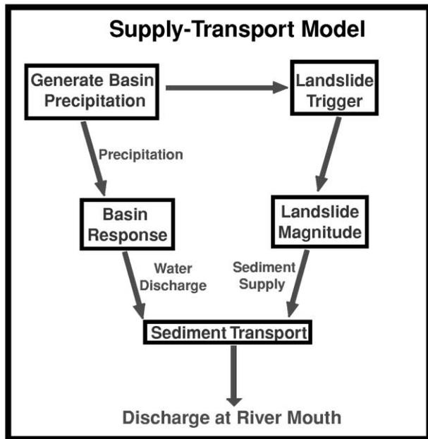
**Figure 6.** Major components of the sediment supply and transport model. See text for details.
