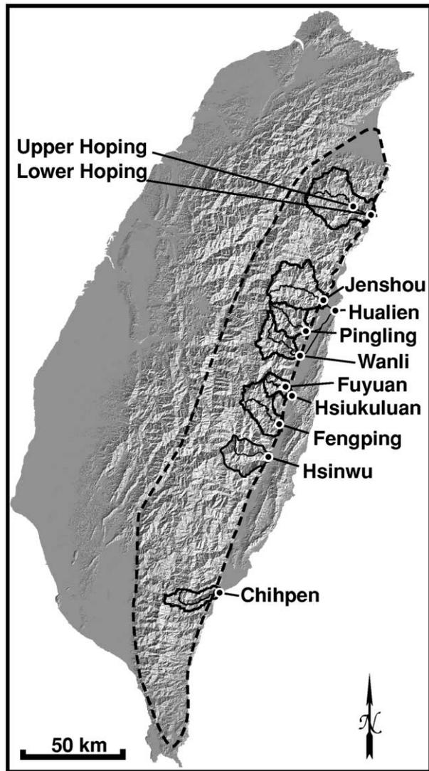
**Figure 1.** Topographic relief map of Taiwan showing location of rivers with basins (*solid lines*) and gauging stations (*dots*) used in this study with the outline of the Central Range (*dashed line*).
